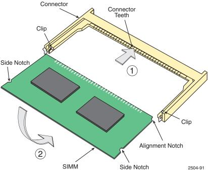
Figure B-3 Installing the DRAM
